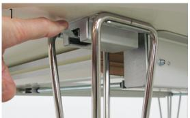
Unlock the extension mechanism by pushing down the levers placed at the end of the guide rails underneath the table top.
